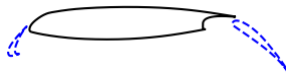
Figure 2: Multi-element airfoil: main body (black solid line), immersed bodies (blue dashed lines)
