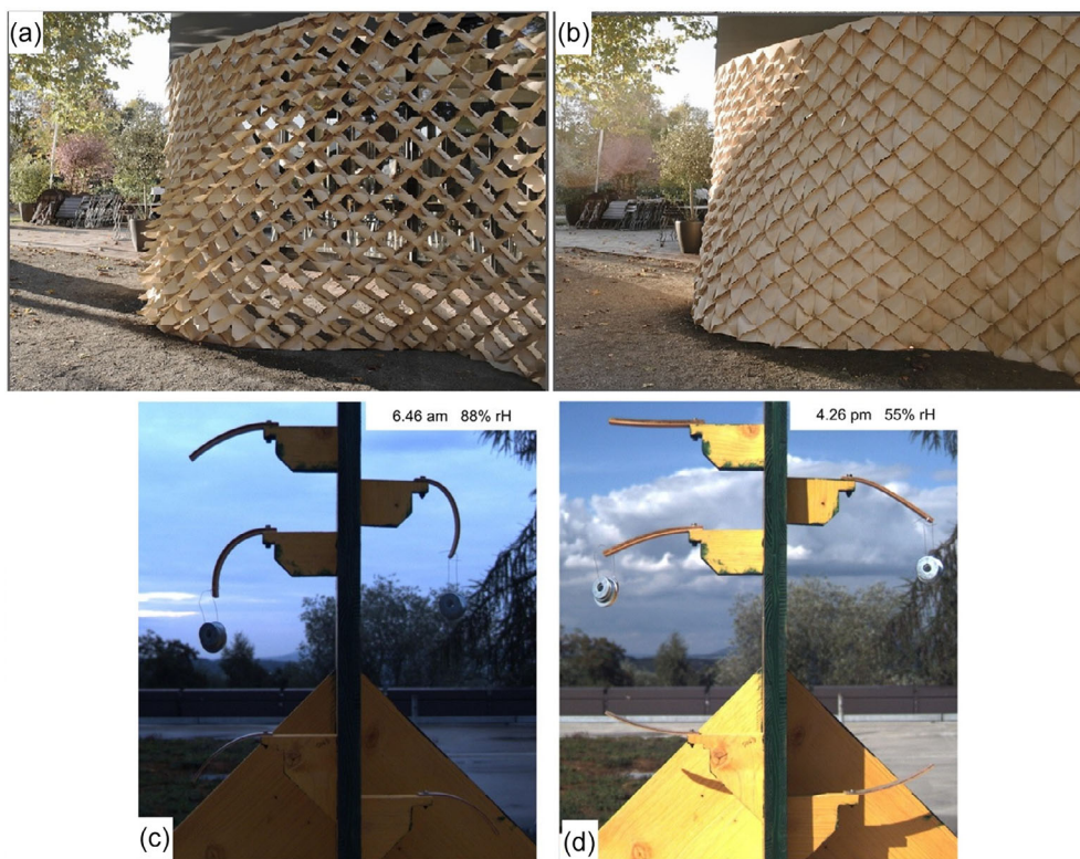
Figure 7. Wood-based actuators at large scale. a) Hygroscope prototype (Reproduced with permission. [119] Copyright 2015, Elsevier) at 40%RH (fully open) and b) at 80%RH (fully closed). c) Curvature response of a bilayer wood actuator at 88%RH and d) 55%RH with attached load under real weather conditions. [102] Taken from the original sources without further modifications.
