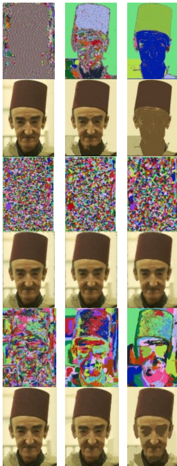
Figure 2: Hierarchies of partition produced at the levels 1, 5, 10 by the quasi-flat-zones (lines 1-2), the non parametric hierarchical watershed (line 3-4) and the nested homogeneous connections (lines 5-6). Segmented images (lines 1-3-5) and their colorized (i.e. mosaic) images (lines 2-4-6).
