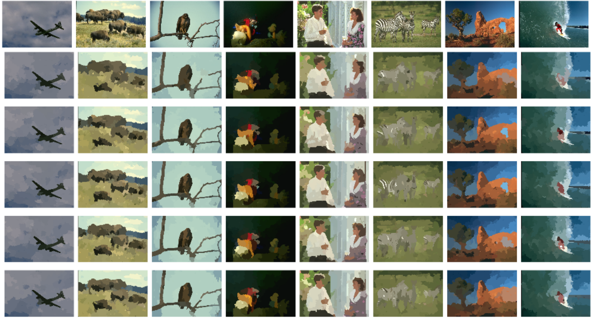
Figure 3. Segmented images with different gradient combinations in Berkeley Segmentation Database and Benchmark (top to bottom : initial image, segmented images (with C=0,2/T=0,8 ; with C=0,5/T=0,5 ; with C=0,7/T=0,3 ; with adaptive combination, with supremum combination)).
