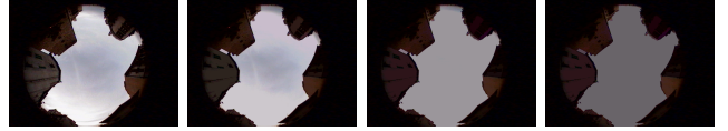
Fig. 4. Geodesic reconstruction according to the contrast parameter H (left to right: original image, GRD with H = 50 , with H = 100 and with H = 150 ).
