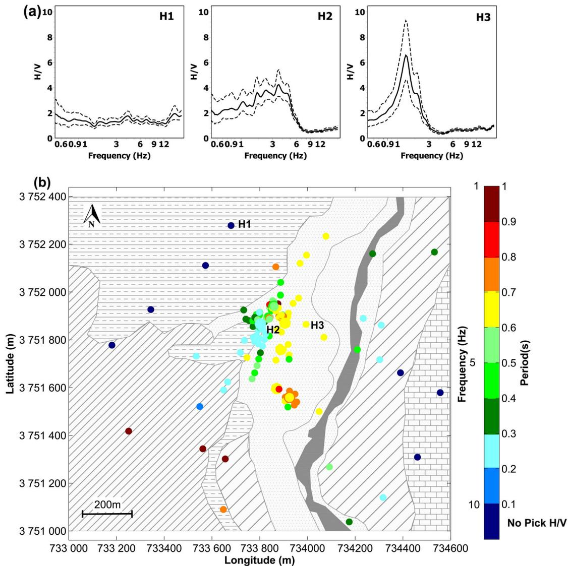
**Figure 8.** (a) Average H/V ratios (thick black line)  $\pm$  standard deviation (dashed black line) at *H1*, *H2* and *H3*, the location of which is indicated in (b). (b) Map of fundamental resonance periods derived from microtremor recordings with the geological units in the background.
