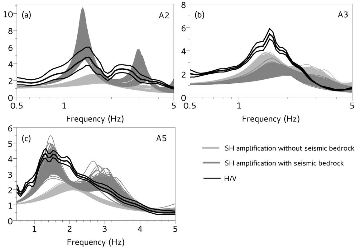
**Figure 16.** Measured average  $H/V$  curves (thick black lines) with related standard deviation (thin black lines) and, theoretical 1D SH transfer functions computed from the ensemble of shear wave velocity profiles shown in Fig. 13. The dark and light grey curves stand for the SH transfer functions computed from the  $V_s$  profiles with and without considering the seismic bedrock.
