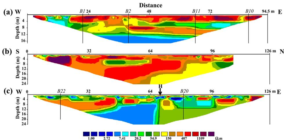
Figure 7. Electrical tomography sections. (a) Electrical profile *E1*, five iterations, Abs error = 4.5 per cent; (b) electrical profile *E2*, 7 iterations, Abs error = 4.7 per cent; (c) electrical profile *E3*, five iterations, Abs error = 6.7 per cent. The profile *E1* was performed on a platform excavated 4 m below the ground level during civil engineering works.
