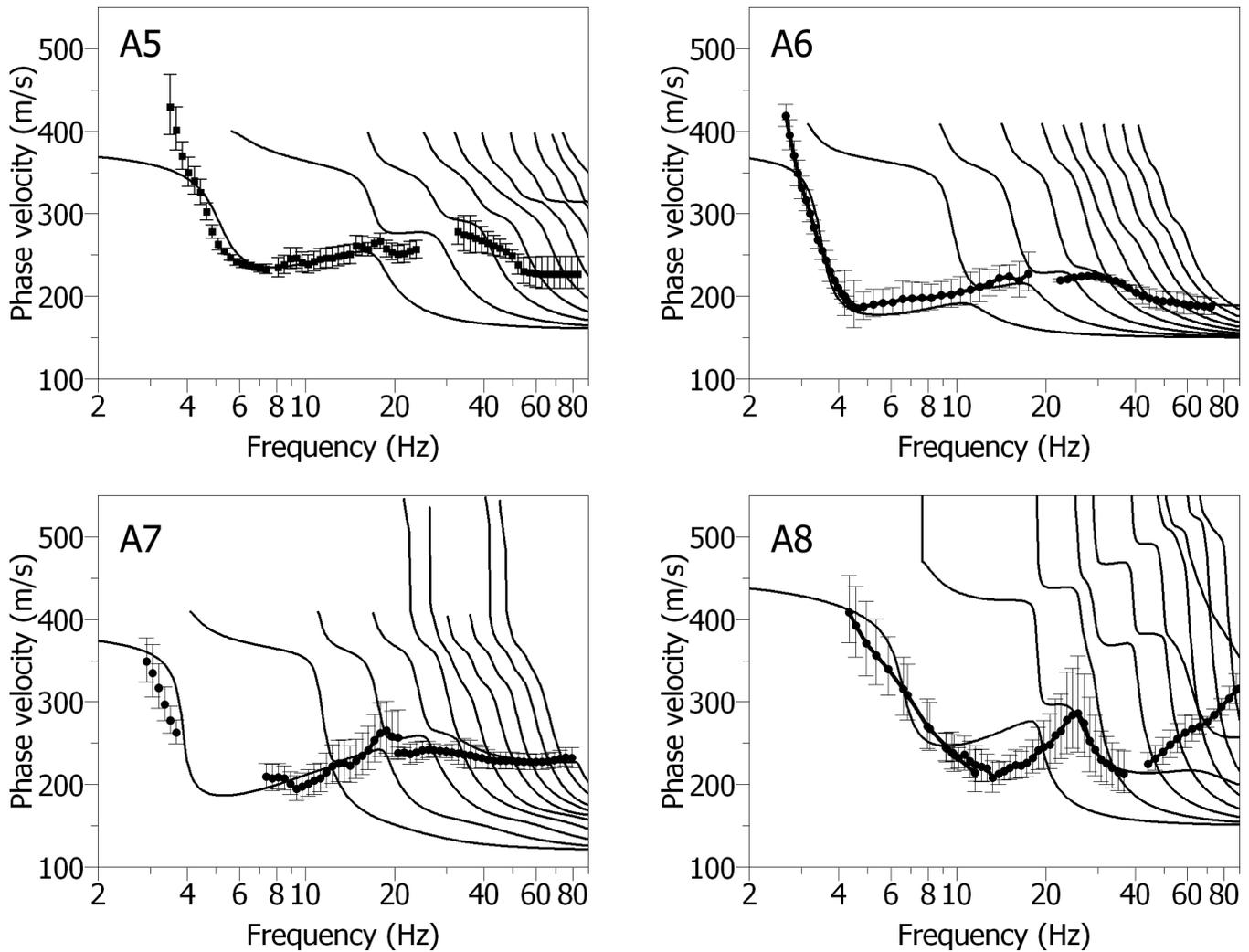
**Figure 12.** Dispersion curve (black dots) measured at arrays *A5–A8*, and theoretical Rayleigh wave dispersion curves for the first ten modes, computed from the simplified velocity structure at boreholes *B20–B23* (Fig. 9), respectively.
