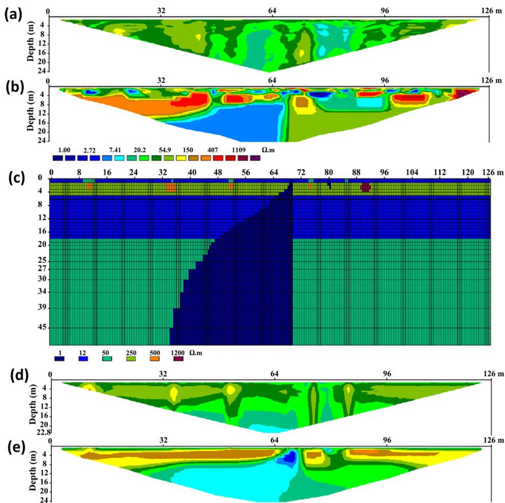
**Figure A1.** (a) Measured pseudosection (E3). (b) Electrical tomography (E3). (c) Synthetic resistivity model of the pollution (see text for details). (d) Pseudosection computed for the synthetic resistivity model. (e) Electrical resistivity tomography obtained for the synthetic model (Abs error = 3.3 per cent after 4 iterations).
