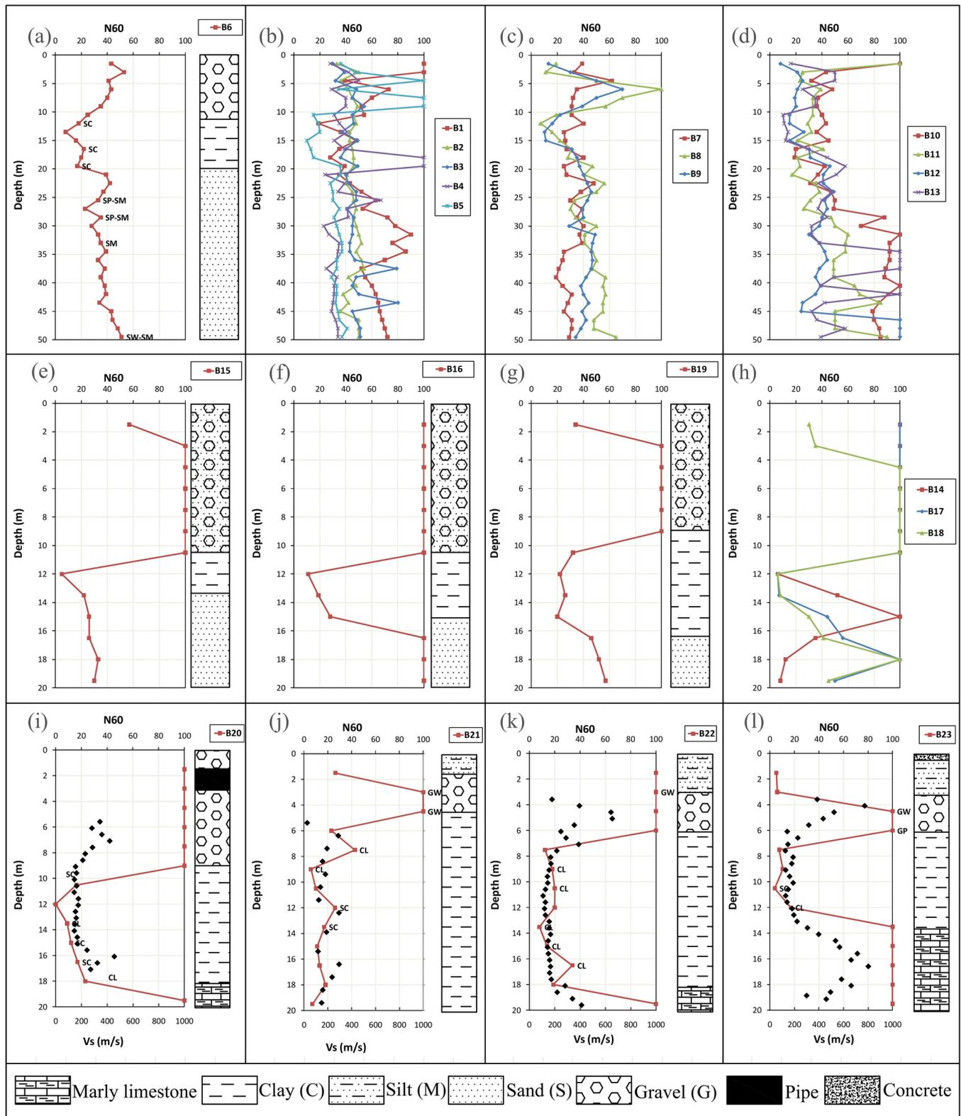
**Figure 5.** SPT profiles and borehole logs at the sites *Si1* (top line: a, b, c and d), *Si2* (middle line: e, f, g and h) and *Si3* (bottom line: i, j, k and l).  $V_s$  values measured during down-hole tests at site *Si3* are plotted for boreholes B20–B23 (i–l). The two-letter symbols of USCS soil classification are indicated when core samples are analysed (CL, low plasticity clay; SC, clayey sand; SM, silty sand; SW, well-graded sand; GW, well-graded gravel; GP, poorly graded gravel).
