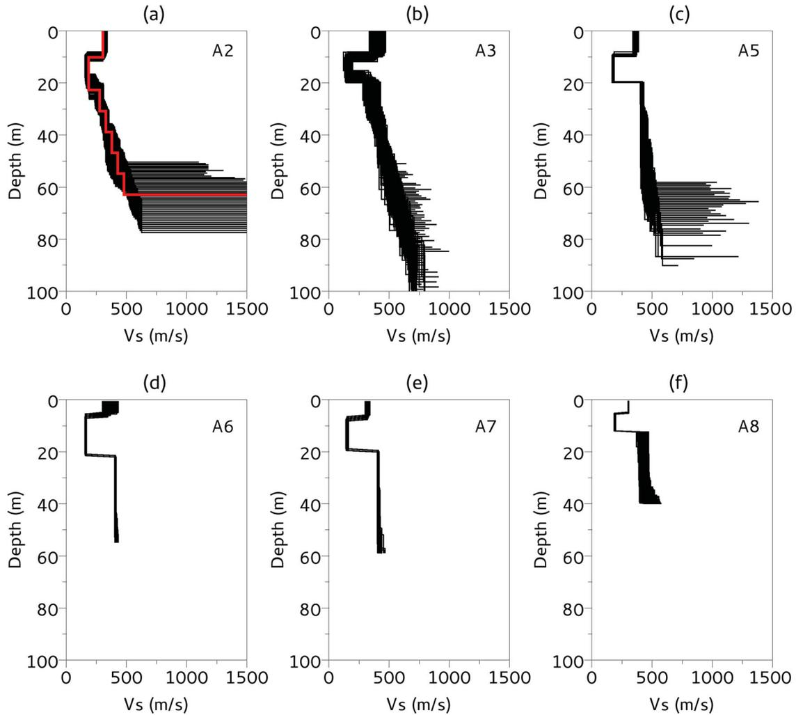
**Figure 13.** Ensemble of inverted shear wave velocity profiles that explain the observed dispersion data within their uncertainty bounds for arrays *A2*–*A8*. The  $V_s$  profile displayed in red for *A2* is used for ambient noise modelling (Fig. 14).
