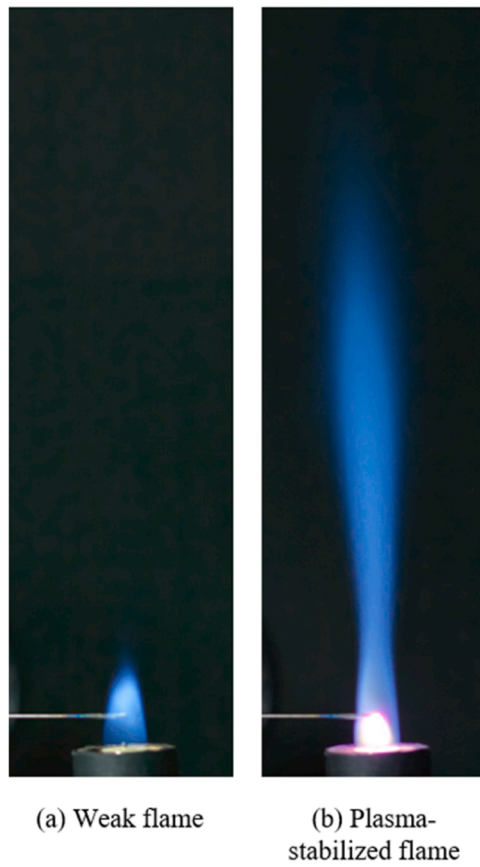
Fig. 2. Photographs in real colors of the lean methane-air flame at \Phi = 0.8 without (a) and with (b) 1.8-mJ NRP discharges applied at 20 kHz. The inter-electrode gap is 5 mm.
