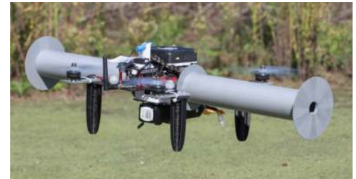
Magnus effect-based quadcopter system
