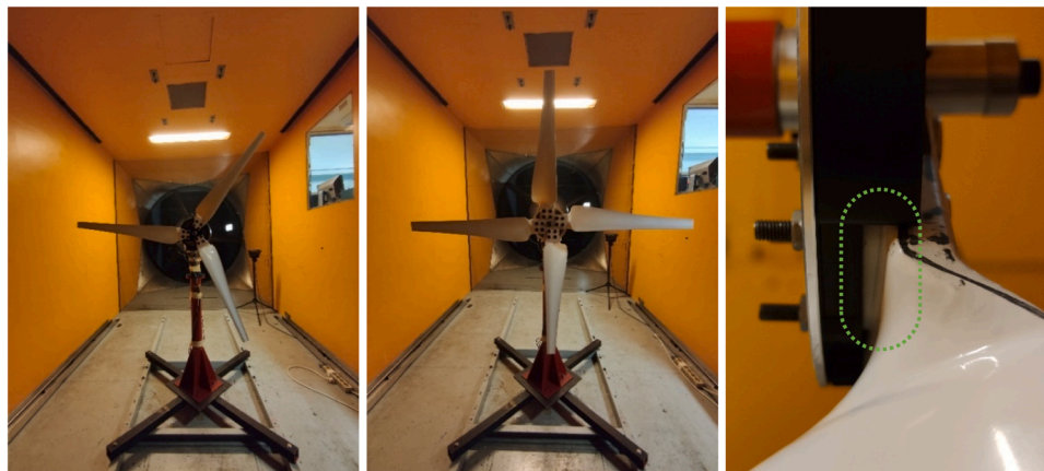
Fig. 5. Wind turbine configuration: (left) 3-bladed rotor, (middle) 4-bladed rotor and (right) pitch modification realised with use of 3D-printed inserts [green] between hub [black] and blade [white].
