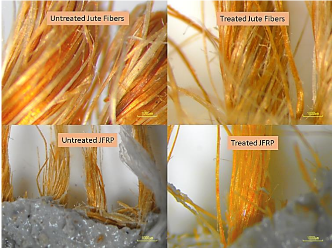
Fig. 3 Microscopic observations on the effect of heat treatment on surface characteristics of jute fibers
