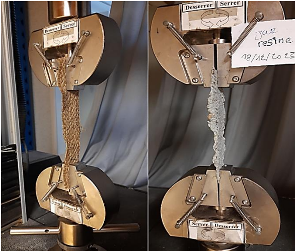
Fig. 4 Experimental setup of tensile strength test of jute fibers and JFRP
