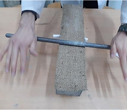
35 36 37 38 39 40 41 42 43 44 45 46 47 Fig. 8 Fiber saturation of resin: full impregnation. 48 49 50 51 52 53 54 55 56 57 58 59 60 61 62 63 64 65
