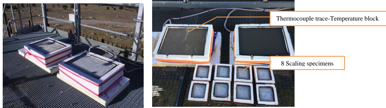
Fig. 3 Concrete blocks instrumented with thermocouples (left), (right) same concrete blocks as well as scaling monitoring specimens, all configured according to the CEN/TS 12390-9 standard.
