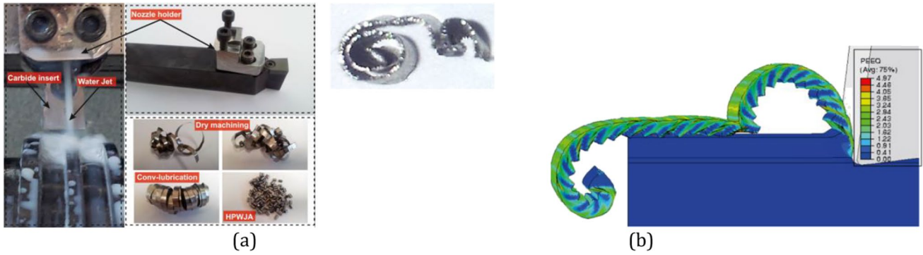
Fig. 10 a Experimental and b numerical chip fragmentation [38]
