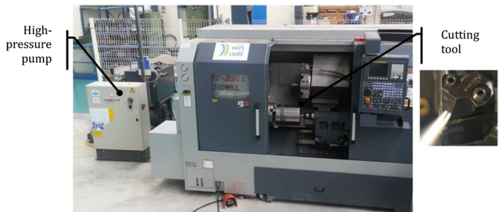
Fig. 3 High-pressure assistance experimental setup (LAMPA)
