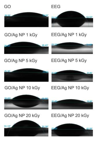
Figure 7. The contact angle of the studied graphene/Ag NPs thin films on polycarbonate membrane.
