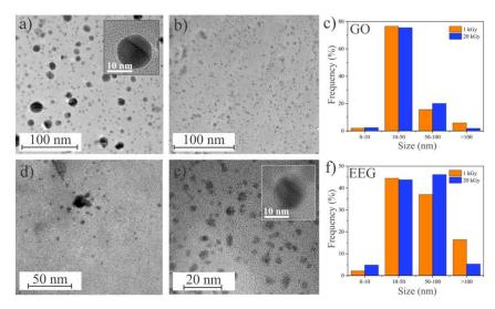
**Figure 3.** TEM images of (a) GO/Ag NPs prepared at 1 kGy irradiation dose, (b) GO/Ag NPs prepared at 20 kGy irradiation dose, (c) particle size distribution for GO/Ag NPs, (d) TEM images of EEG/Ag NPs prepared at 1 kGy irradiation dose, (e) EEG/Ag NPs prepared at 20 kGy irradiation dose and (f) particle size distribution for EEG/Ag NPs.
