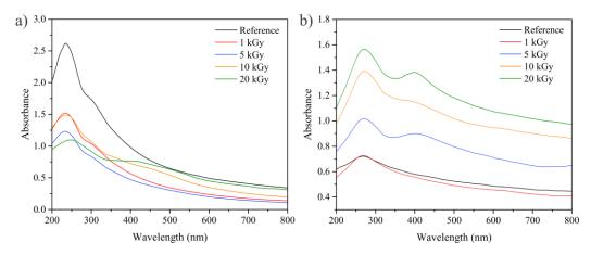
**Figure 6.** UV–Vis spectra of (a) GO (reference) and GO/Ag NPs prepared at different irradiation doses and (b) EEG (reference) and EEG/Ag NPs prepared at different irradiation doses.
