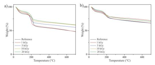
**Figure 5.** TGA curves of (a) GO (reference) and GO/Ag NPs prepared at different irradiation doses and (b) EEG (reference) and EEG/Ag NPs prepared at different irradiation doses.
