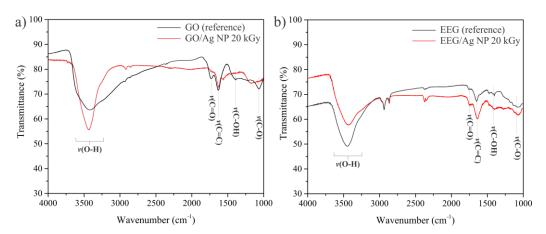
**Figure 2.** FTIR spectra of (a) GO (reference) and GO/Ag NP composite irradiated at 20 kGy and (b) EEG (reference) and EEG/Ag NP composite irradiated at 20 kGy.
