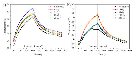
**Figure 8.** The temperature changes induced by a 532 nm laser irradiation for (a) GO (reference) and GO/Ag NPs prepared at different irradiation doses and (b) EEG (reference) and EEG/Ag NPs prepared at different irradiation doses.
