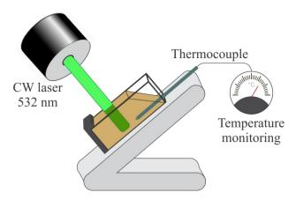
Figure 1. Experimental setup for the photothermal efficiency measurements.
