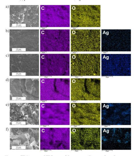
**Figure 4.** SEM image and EDS maps of the corresponding area for carbon, oxygen, and silver for (a) GO, (b) GO/Ag NPs prepared at 5 kGy, (c) GO/Ag NPs prepared at 20 kGy, (d) EEG, (e) EEG/Ag NPs prepared at 5 kGy, and (f) EEG/Ag NPs prepared at 20 kGy.
