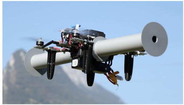
Fig. 1: Magnus-effect winged quadcopter system (MWQ). The gray cylinders are the Magnus-effect based wings. The quadcopter's four rotors are attached to the arm extensions. A short video of one of the outdoor experiments is available at <https://youtu.be/dtGctfuA6s>
