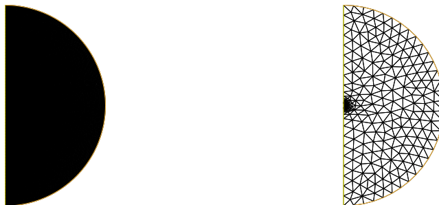
Figure 7: Left: reference mesh used for simulating the Transport-Stokes equation in \mathbb{R}^3 , in an axisymmetric setting, using artificial boundary conditions on the boundary of the truncated domain. Right: initial computational mesh, adapted to \rho_0 .
