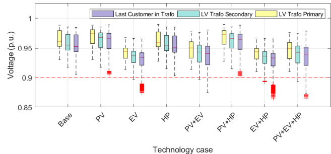
Fig. 8: Voltage measured at different points for all transformers and each case
