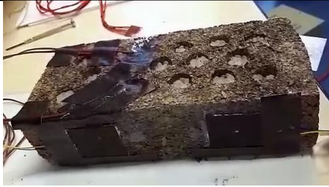
Figure 7c: View of the brick with holes filled by PCM.
