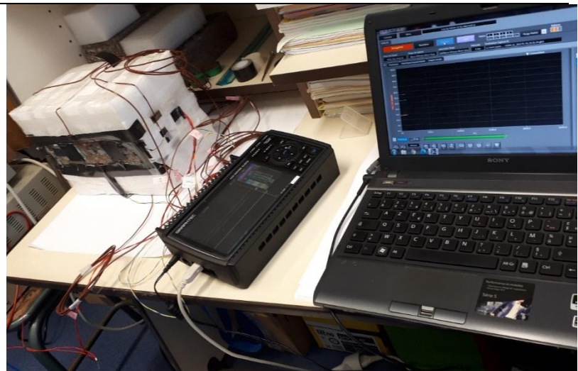
Figure 7b: All the equipment making up the experimental measurement chain: sample, acquisition unit and computer.
