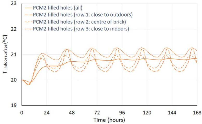
Figure 23: simulated temperature evolution of the indoor surface of the 1-layer brick wall filled with PCM2 (all, row1, row2 or row3), exposed to an outdoor temperature fluctuation and an outdoor radiation flux.
