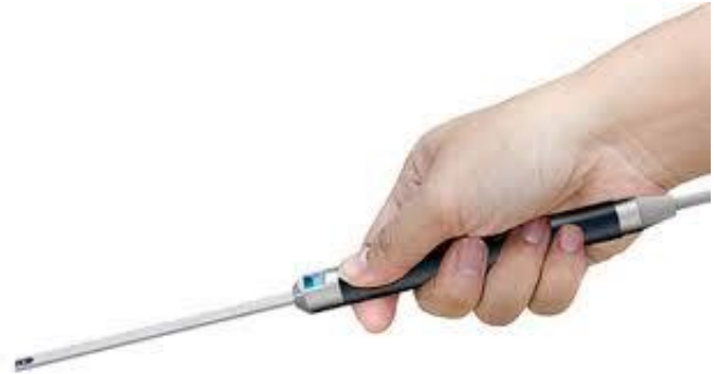
Fig.2. Illustration of use of a Hall probe sensor.
