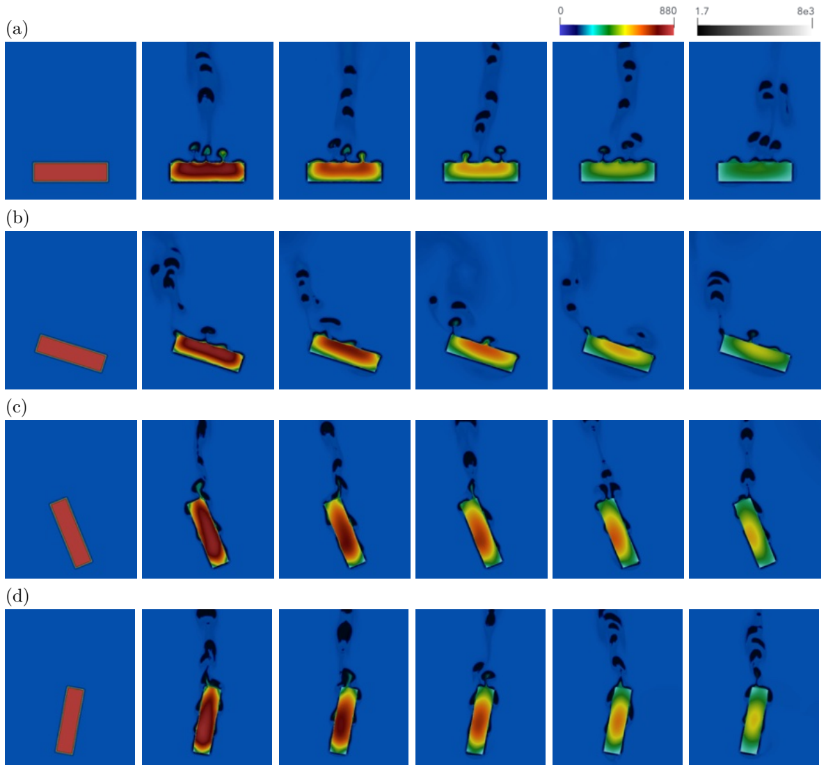
Figure 13: Temperature evolution for the rectangular brick test case inserted at various angles. (a) \theta = 0^\circ , (b-d) random angles selected over the course of optimization, and (e) \theta = 97^\circ , the optimal angle selected by the DRL agent. The snapshots are sampled (from left to right) every 10s from 0 to 50s. The iso-contours in the solid (resp. in the fluid) show the temperature field between 0 and 880^\circ\text{C} (resp. the density field between 1.7 and 8000\text{ kg/m}^3 ).
