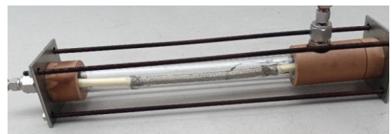
Fig. 1 Diagram and photograph of the air-tight ageing chamber containing a cable sample.
