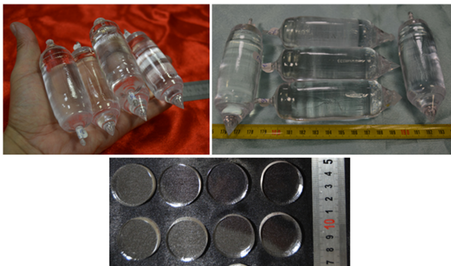
Fig. 3 Top: Picture of the sapphire crystals grown under a stationary stable regime. Bottom: Different samples of 15 mm thick cylinder prepared from sapphire ingot.
