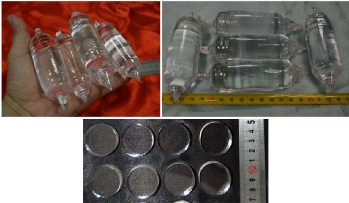
Figure 3: Top: picture of the sapphire crystals grown under stationary stable regime. Bottom: different samples of 15 mm thick cylinder prepared from sapphire ingot
