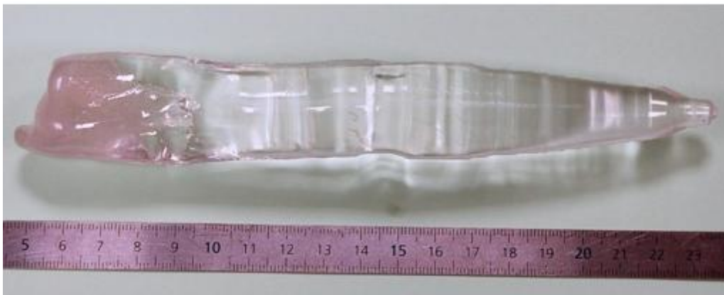
Figure 2: Sapphire ingot grown without automatic program showing diameter instability.
