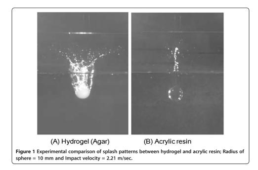
surface conditions of the solid object. It is noted that the fact that the forms of splash caused by a solid sphere with the same weight and the same diameter differ according to the surface condition is not known in general.
