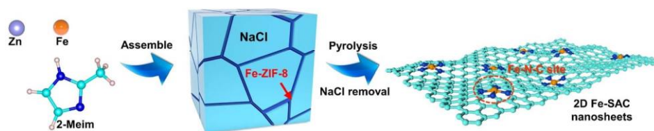
Scheme 1 Schematic illustration of the synthetic procedures for 2D Fe single-atom catalysts.
