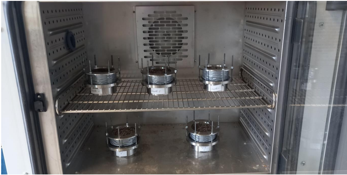
Figure 1 : S/BP samples having their sides sealed with waterproof aluminum tape and fixed at top of cups enclosing a solution of potassium nitrate (KNO 3 ) at their bottoms
