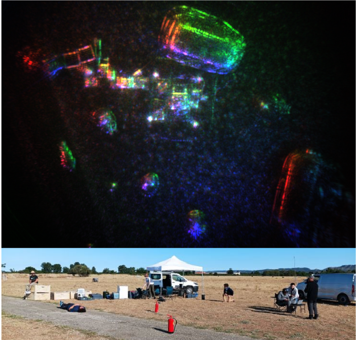
Fig. 4. Concatenation of SAR images measured while the drone was performing a circle around the scenery. Each color corresponds to a different illumination direction. One can identify on top of the image the car visible at the back of the photo, as well as the four poles of the tent in the center and the sleeping man at the left-hand-side. Red comes roughly from the top left, green from the top right and blue from the bottom of the image.
