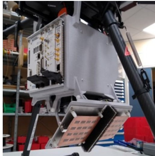
Fig. 1. The SAR tool embedded under the UAV. The structures holding the RF parts and the antennae are 3D printed. The antenna needs to be oriented manually.
