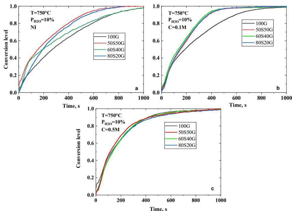
**Figure 2.** Conversion level versus time for all biomasses: (a). Non-impregnated biomasses; (b). Impregnated biomasses with  $C = 0.1$  M; (c). Impregnated biomasses with  $C = 0.5$  M.
