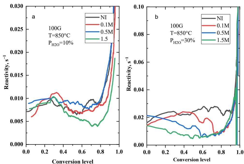
Figure 9. (a) Reactivity profile of 100G versus conversion with 10% H<sub>2</sub>O and (b) with 30% H<sub>2</sub>O.
