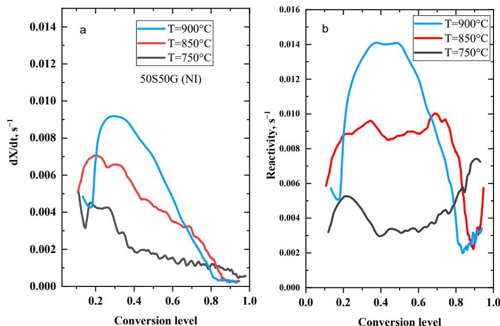
Figure 7. (a) Reaction rate as a function of conversion for 50S50G at different temperatures with 10%  $H_2O$  and (b) Reactivity versus conversion for the same sample.
