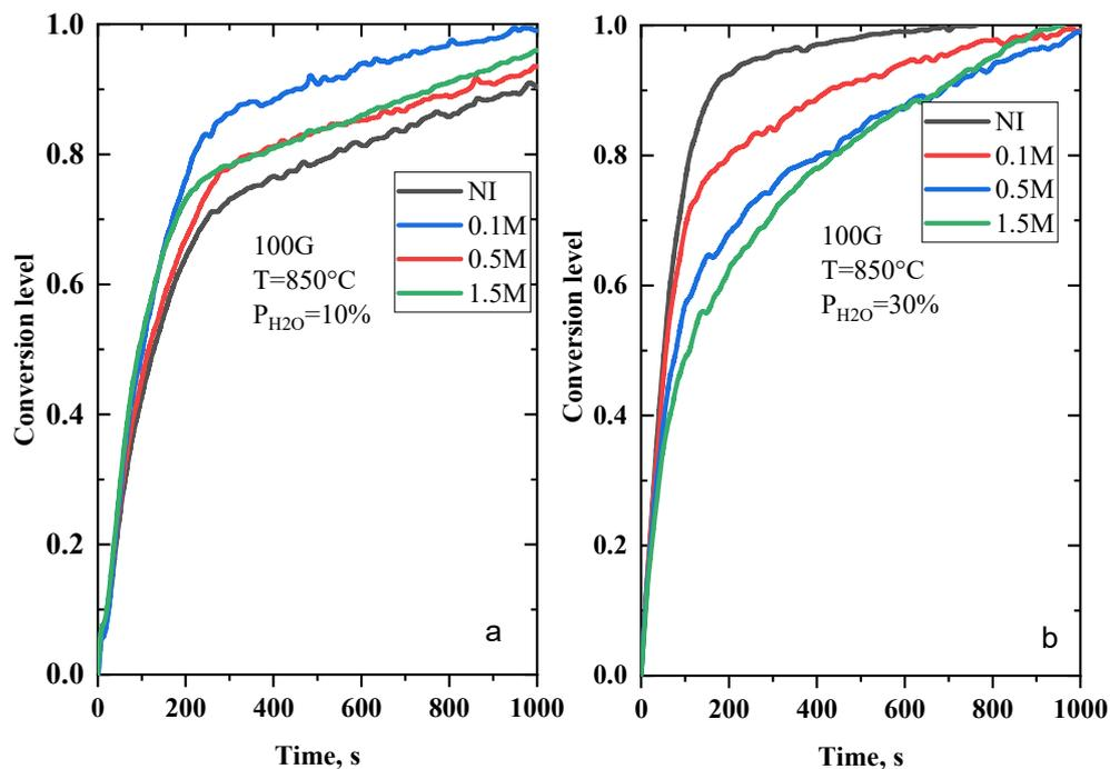
Figure 8. (a) Conversion versus reaction time for 100G with 10% H<sub>2</sub>O and (b) with 30% H<sub>2</sub>O.
