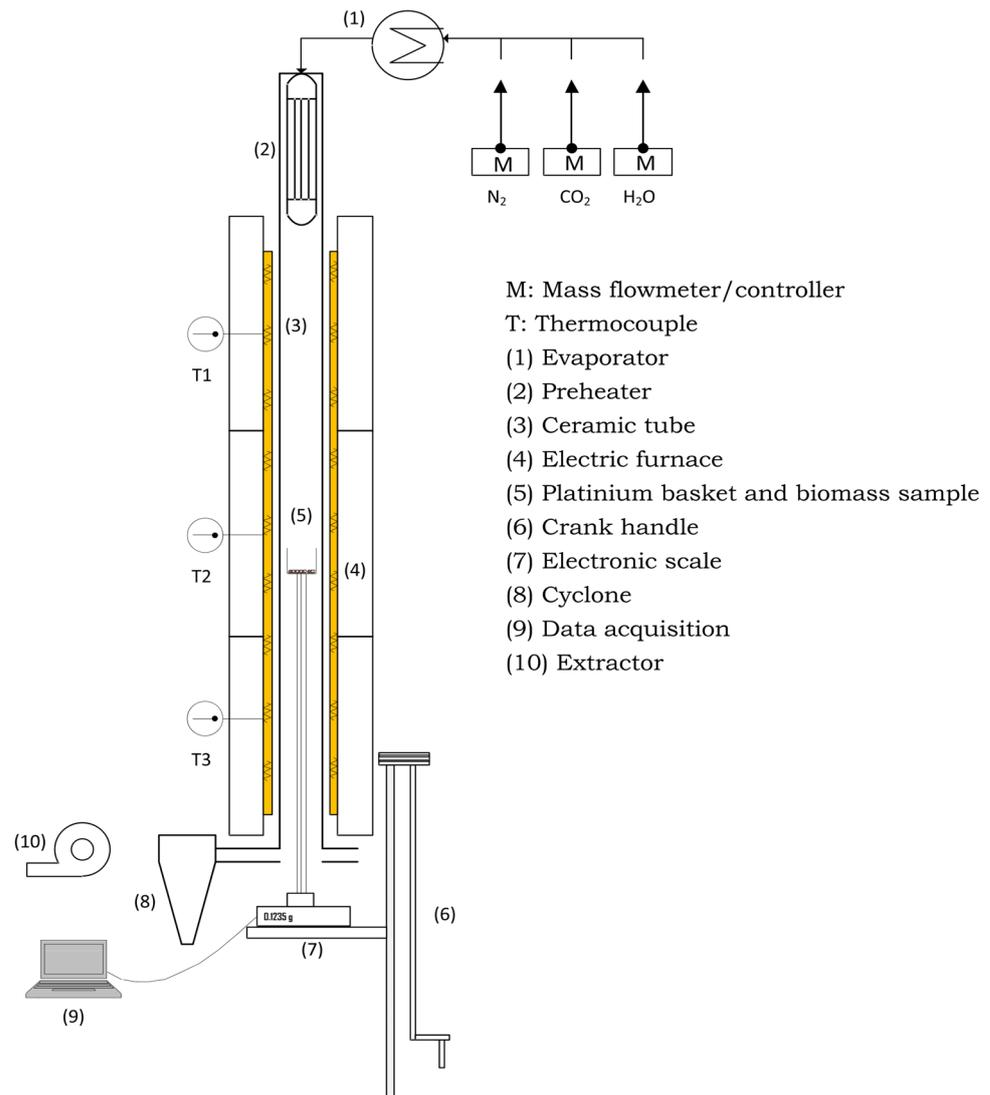
**Figure 1.** Schematic representation of the M-TG reactor [32].
