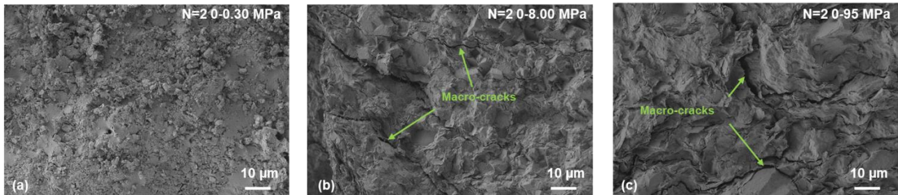
Figure 2. SEM pictures from specimens exposed to 2 wetting and drying cycles with different ranges of suctions.
