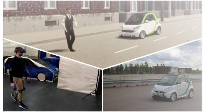
Fig. 9: AEB testing in a MR environment [73].
