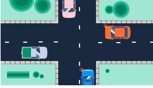
Figure 11: In this configuration, if all the cars want to go straight ahead but respect the rule “right of way” rule, the situation will remain eternally blocked. The same applies if all cars decide to ignore the rule and pass at the same time (crash). But if just one “aggressive” car forces its way through while the others stay “passive”, the situation will be unblocked. Having different behavior can help to solve conflict.
