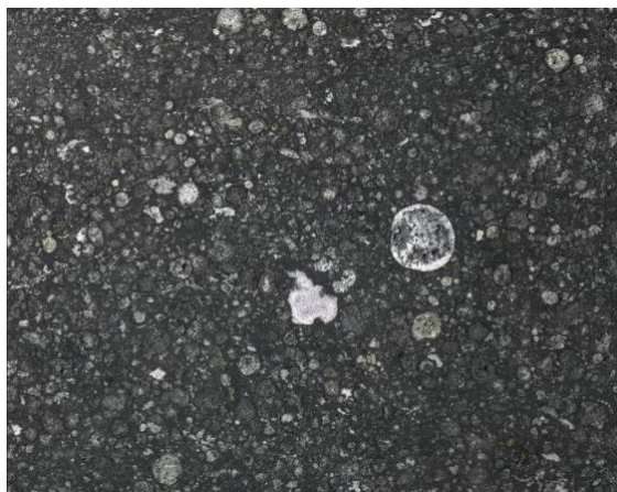
Figure 3: Polished section ( \sim 6.5 \times 4.5 cm) of the Allende CV3.6 carbonaceous chondrite meteorite, which fell on February 8th, 1969 in Mexico. The total known recovered mass is \sim 2 tons. Allende comprises a fine-grained ( < 100 mm) matrix of dark primary and secondary silicates, oxides, and opaque minerals, and lithic clasts such as chondrules (rounded vitreous objects), abundant refractory inclusions found as calcium-aluminum-rich inclusions (CAIs, white objects with various shapes) or ameboid olivine aggregates (AOAs), and dark inclusions. The matrix also contains abundant organic matter and circumstellar condensates (not visible at this scale). Credit: Laurence Garvie (ASU).
