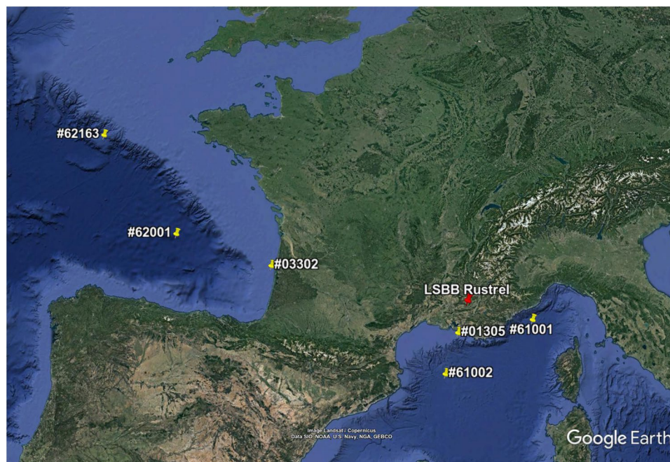
Figure 1. Buoys' locations and LSBB. The site of interest used to validate the forecast protocol, the LSBB, is indicated with a red icon. Yellow thumbtacks with NOAA ID codes show the 6 buoys considered for the seismic noise forecasts. Image generated with Google Earth™ mapping service. Map Data: Image Landsat / Copernicus, Data SIO, NOAA, U.S. Navy, NGA, GEBCO.
