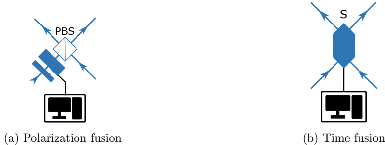
Figure 15: (a) Fusion station for polarization qubits. The transformation required is that of a polarized beam splitter (PBS). (b) Fusion station for time bin entanglement, done by an intensity modulator.
