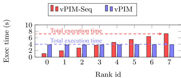
Figure 16: Execution time of virtio requests for a write-to-rank operation across 8 ranks. In the non-parallel version (red), requests are processed sequentially in the backend, while in the multithreaded version (blue), they are handled in parallel.
