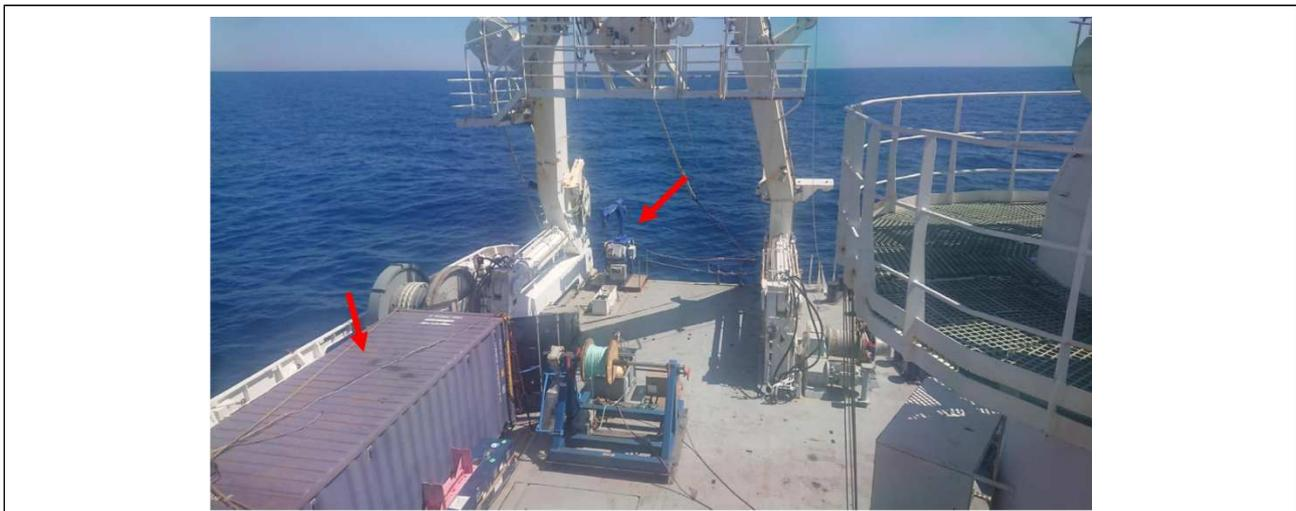
Figure 19. MVP200 (winch and container) installation on the deck.
