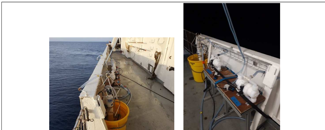
Figure 44. Pumping system deployed during the BioSWOT-Med cruise composed of two AstiPure pumps, two PE tubes (50 and 26 m long in the water) and a Seabird SBE19+ CTD .
