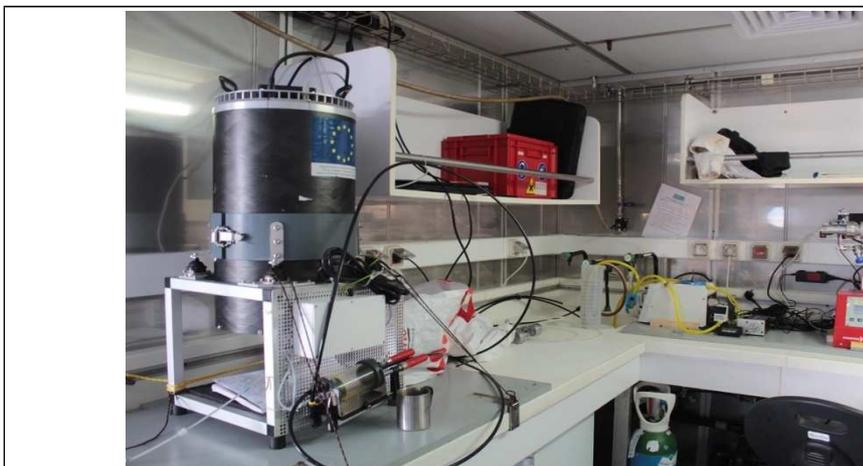
Figure 22. The shipboard setup of the automated flow cytometry platform.
