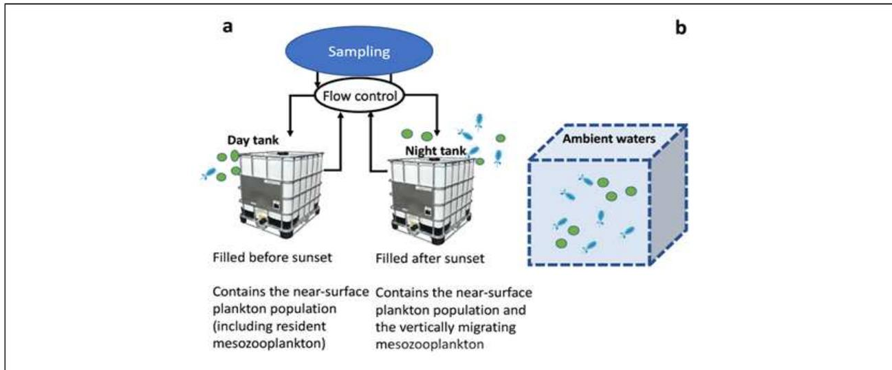
Figure 50. Schematic of the key concept behind the mesocosm experiment.
