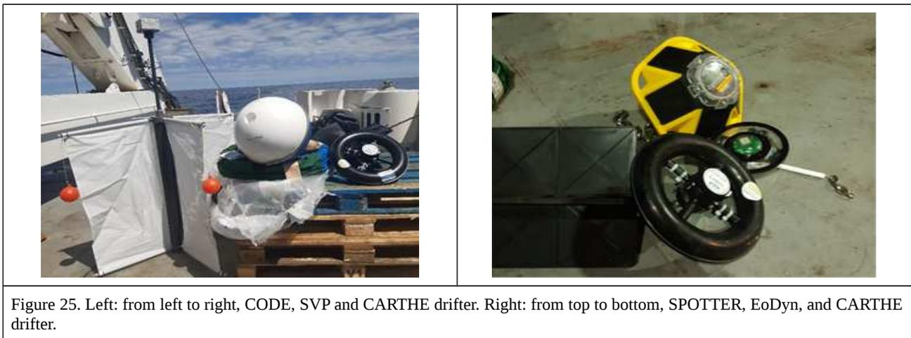
Figure 25. Left: from left to right, CODE, SVP and CARTHE drifter. Right: from top to bottom, SPOTTER, EoDyn, and CARTHE drifter.
