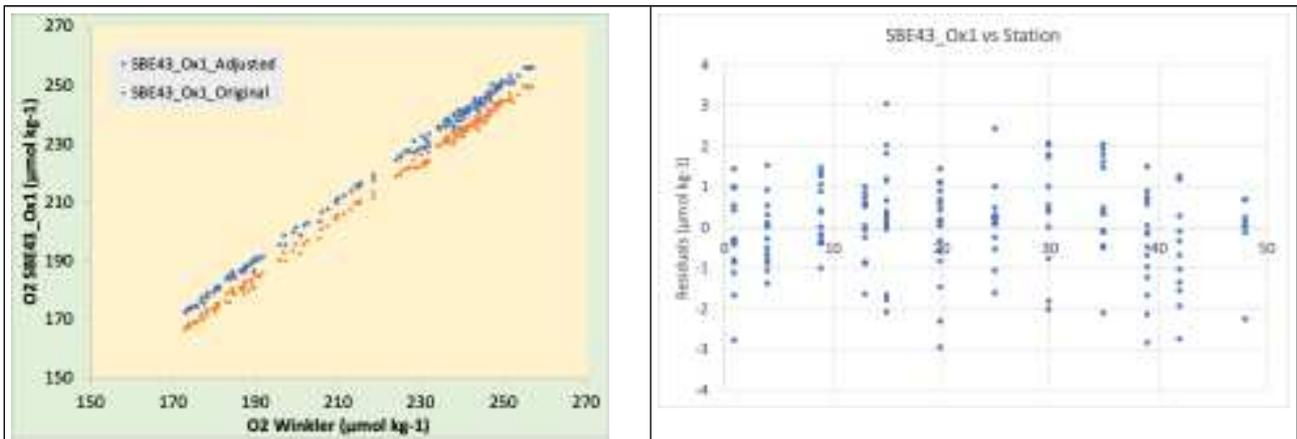
Figure 42. Left: Relationship between the O2 values of the SBE43 sensor before and after correction as a function of the oxygen measured by the Winkler method ( $\mu\text{mol O}_2 \text{ kg}^{-1}$ ). Right: Distribution of residuals ( $\text{O}_2\text{SBE43}$  minus  $\text{O}_2\text{W}$ ) as a function of station number.
