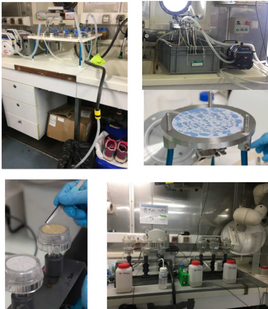
Figure 46. Genomics platform on board R/V L'Atalante. Top: The tripods installation for Niskin and underway water filtration. Bottom: the filtration ramp for the net tows' samples.
