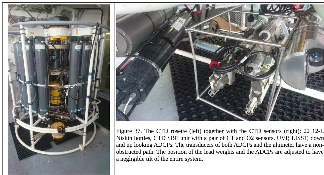
Figure 37. The CTD rosette (left) together with the CTD sensors (right): 22 12-L Niskin bottles, CTD SBE unit with a pair of CT and O2 sensors, UVP, LISST, down and up looking ADCPs. The transducers of both ADCPs and the altimeter have a non-obstructed path. The position of the lead weights and the ADCPs are adjusted to have a negligible tilt of the entire system.
