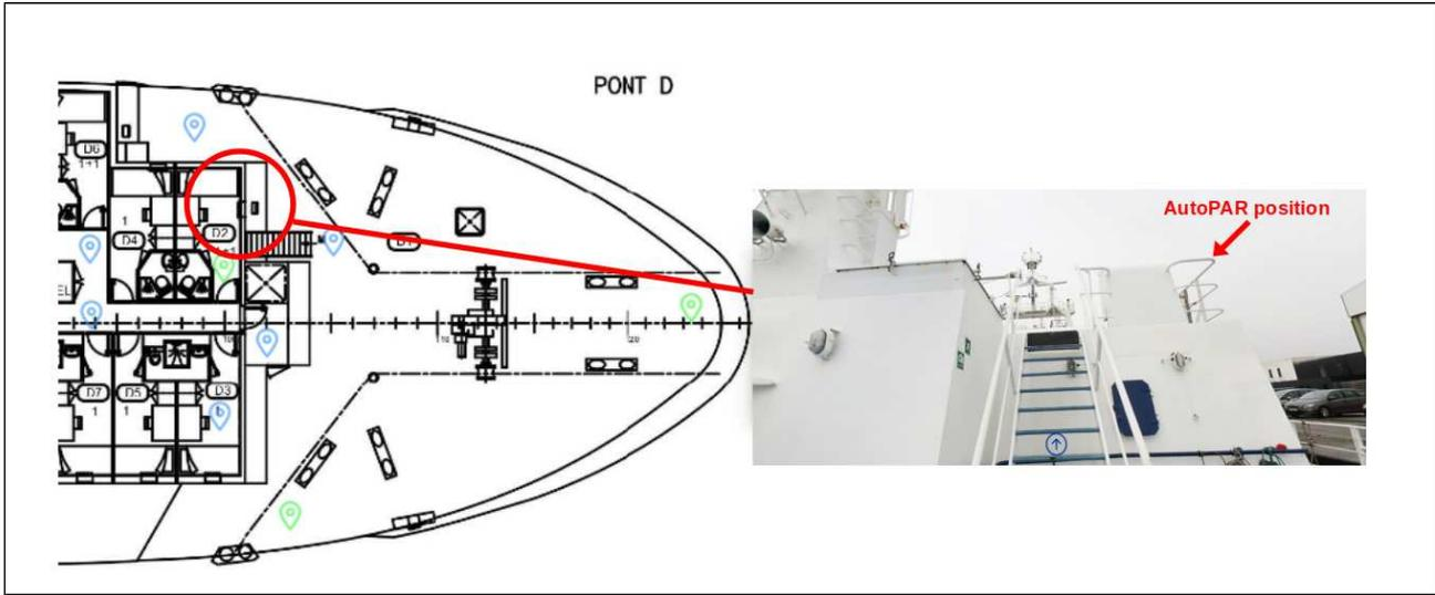
Figure 19: Position of the AutoPAR sensor.
