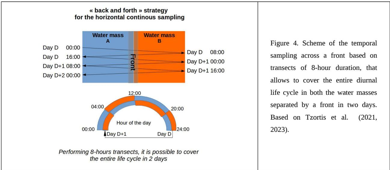
Figure 4. Scheme of the temporal sampling across a front based on transects of 8-hour duration, that allows to cover the entire diurnal life cycle in both the water masses separated by a front in two days. Based on Tzortis et al. (2021, 2023).
