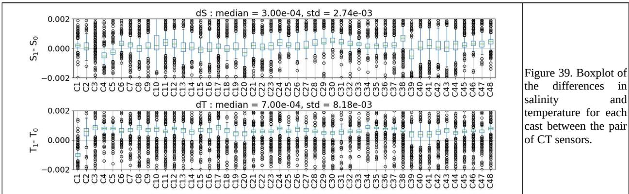
Figure 39. Boxplot of the differences in salinity and temperature for each cast between the pair of CT sensors.
