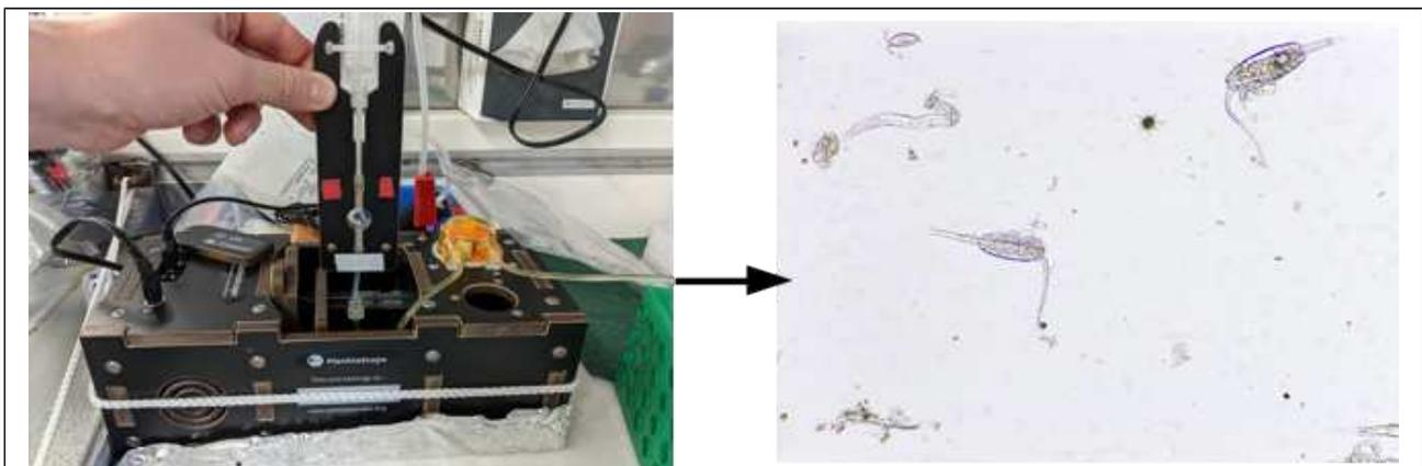
Figure 49. Planktoscope and an example of image obtained.
