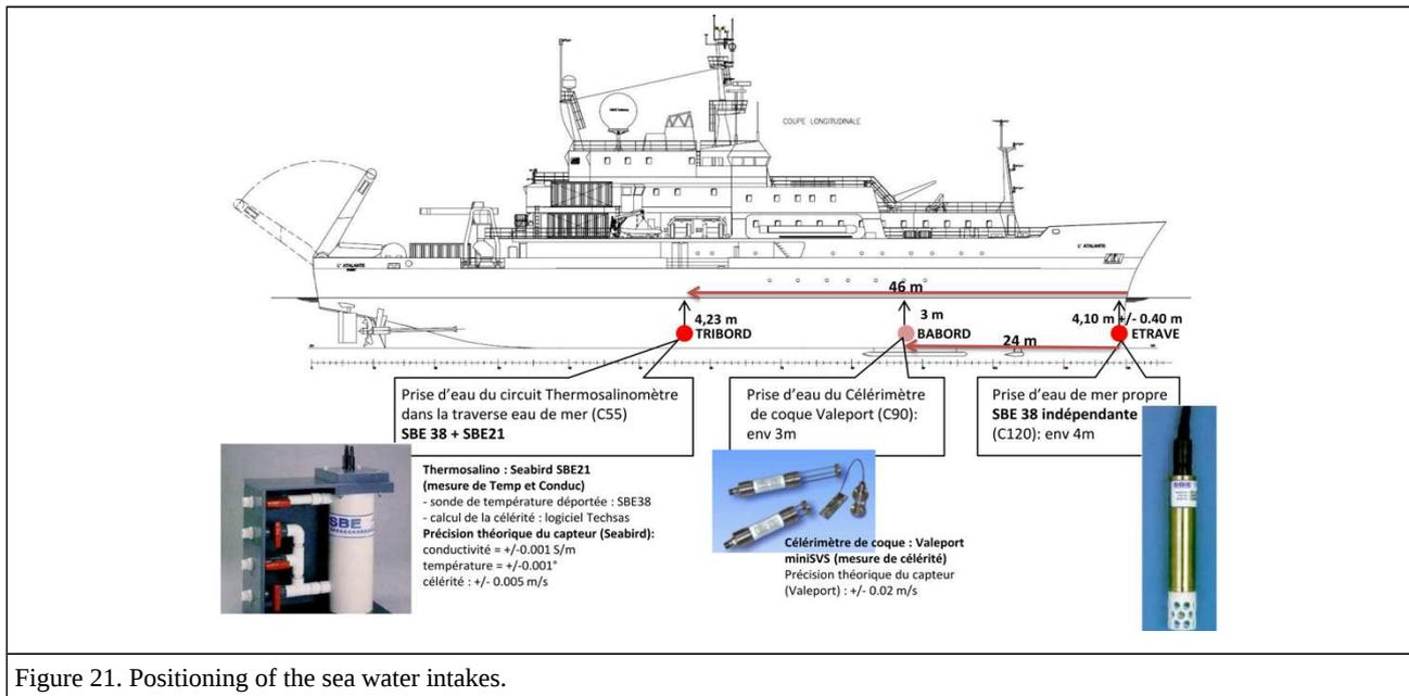
Figure 21. Positioning of the sea water intakes.
