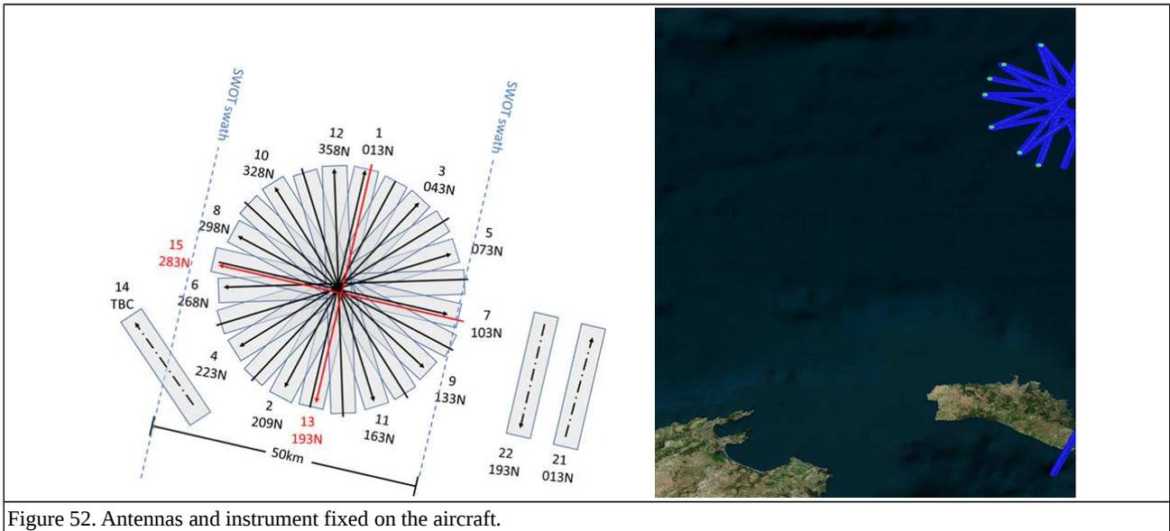
For this campaign we proceeded with 3 flights on the 5, 7 and 8 May when wind conditions were strong enough for the radar to get enough backscattered signal. The same acquisition pattern was proceeded for the three days with a rose pattern within a disk of about 50km in diameter centered at 41.09°N, 4.29°E (see Figure 52). A calibration track over the East part of Minorca was proceeded at the beginning of each flight.
