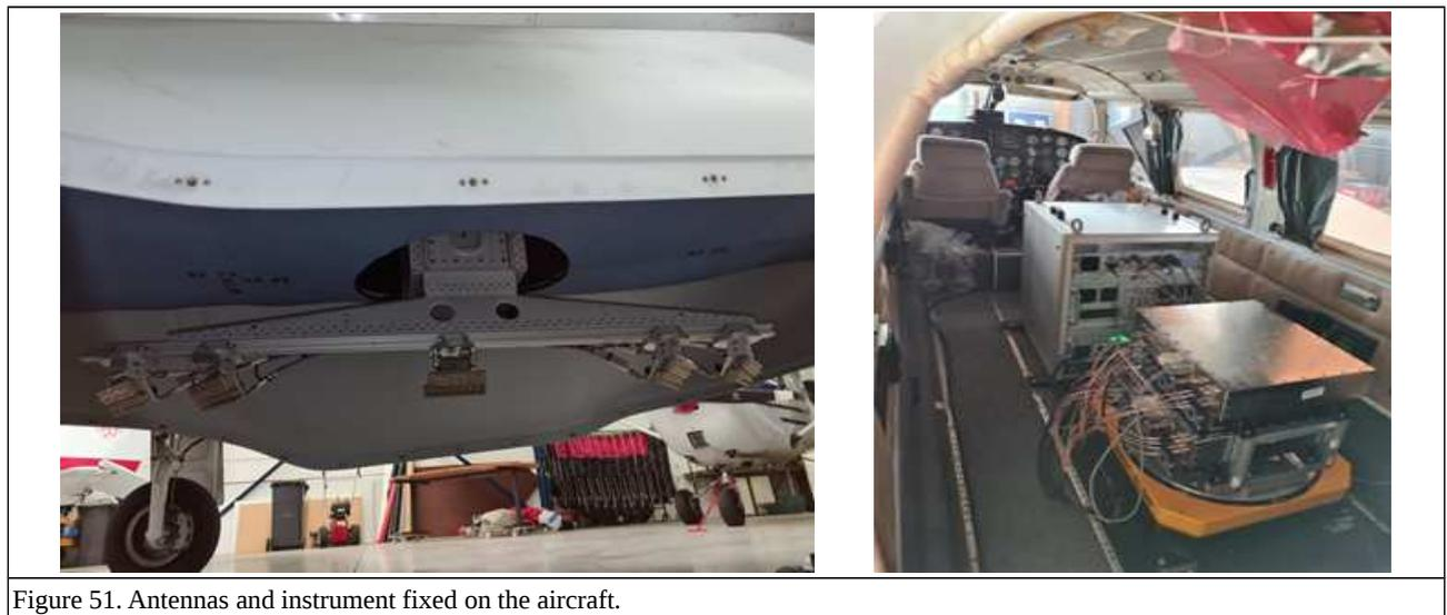
Figure 51. Antennas and instrument fixed on the aircraft.
