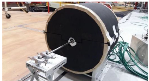
Fig. 12 Positioning of neutron sources inside the LOENIEv2 detector for efficiency calibration
