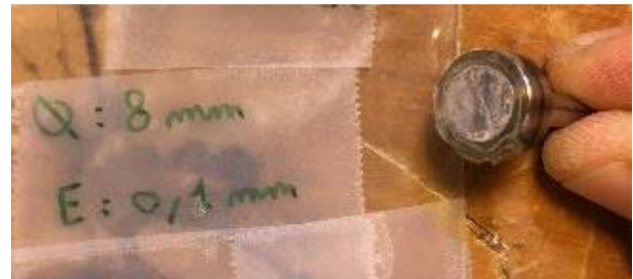
Fig. 16 Photo of the Al-Au activation foil for neutron flux calibration
