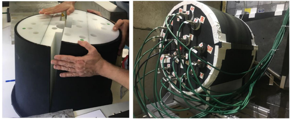
Fig. 3 LOENIEv2 long counter, during the assembling of the HDPE matrix (left-side) and final installation in the PF1B experimental area (right side)
