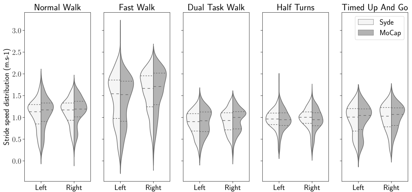
Figure 12. The horizontal stride velocity distributions, computed from the inertial sensor and the motion capture ground truth, for each ankle, for all five exercises.
