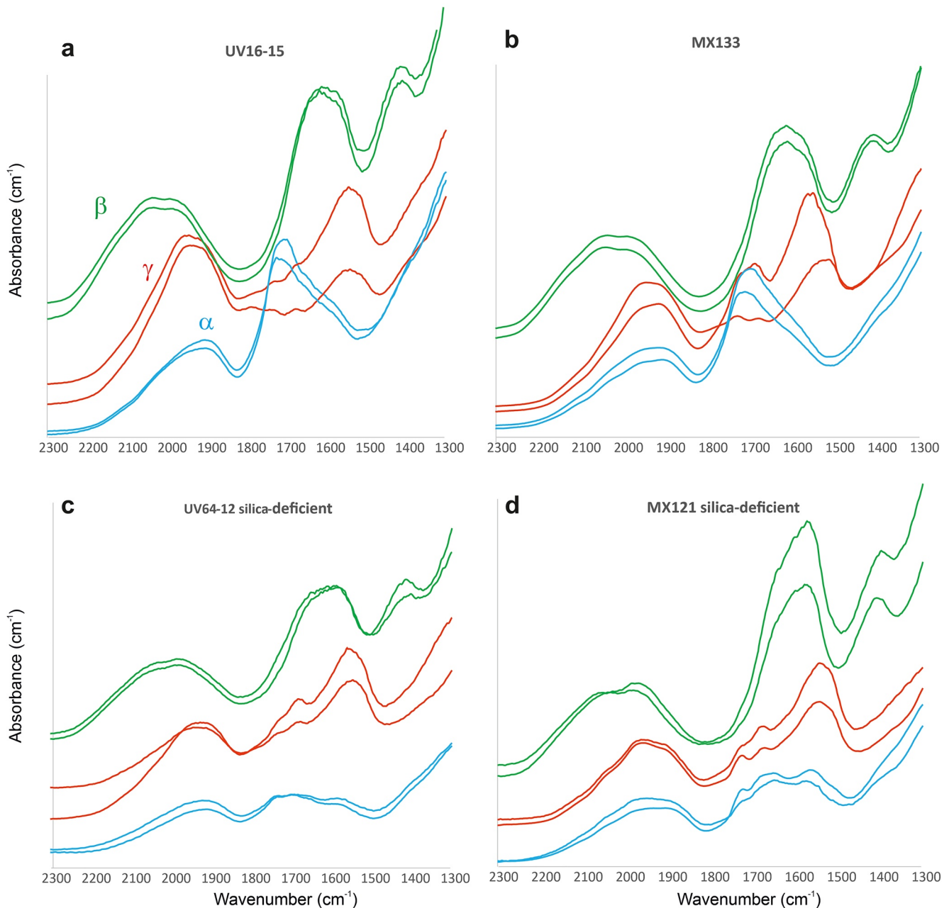
Figure 2. Typical Fourier Transform Infrared Spectroscopy absorption bands related to lattice overtones for clinopyroxene in four eclogite xenoliths from the Siberian and Slave cratons.
