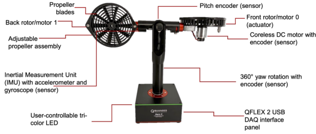
Figure 1: Quanser Aero : 2 degree of freedom configuration [image by Quanser Inc.]
