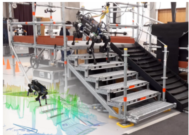
Figure 1. Industrial staircase descent with onboard perception. Video: https://youtu.be/bNVxTh0eixI .
