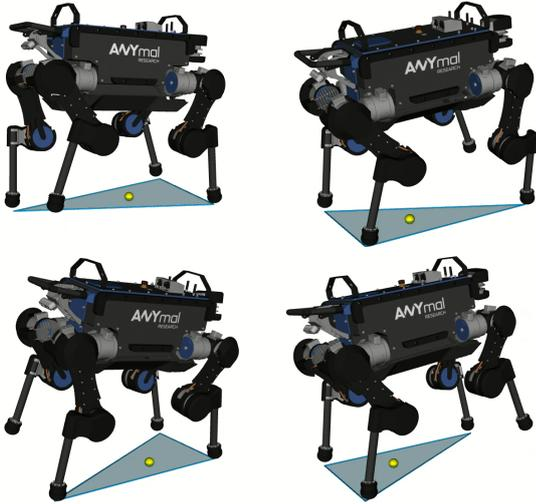
**Figure 14.** Screenshots of the motion resulting from our OCP regularization setup for a walking gait pattern. The blue area between represents the support polygon and the yellow circle is the Centre Of Pressure (COP) applied.
