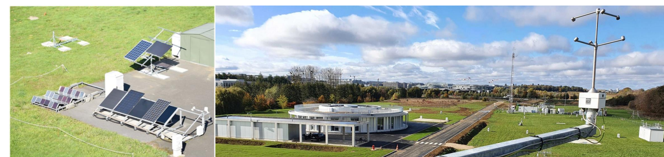
SIRTAs platform PV panels in real conditions with environmental measurement facilities
