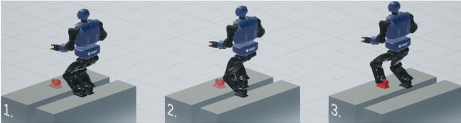
Fig. 1: A footstep sequence allowing to reach the target position for the left foot in 2 steps.
