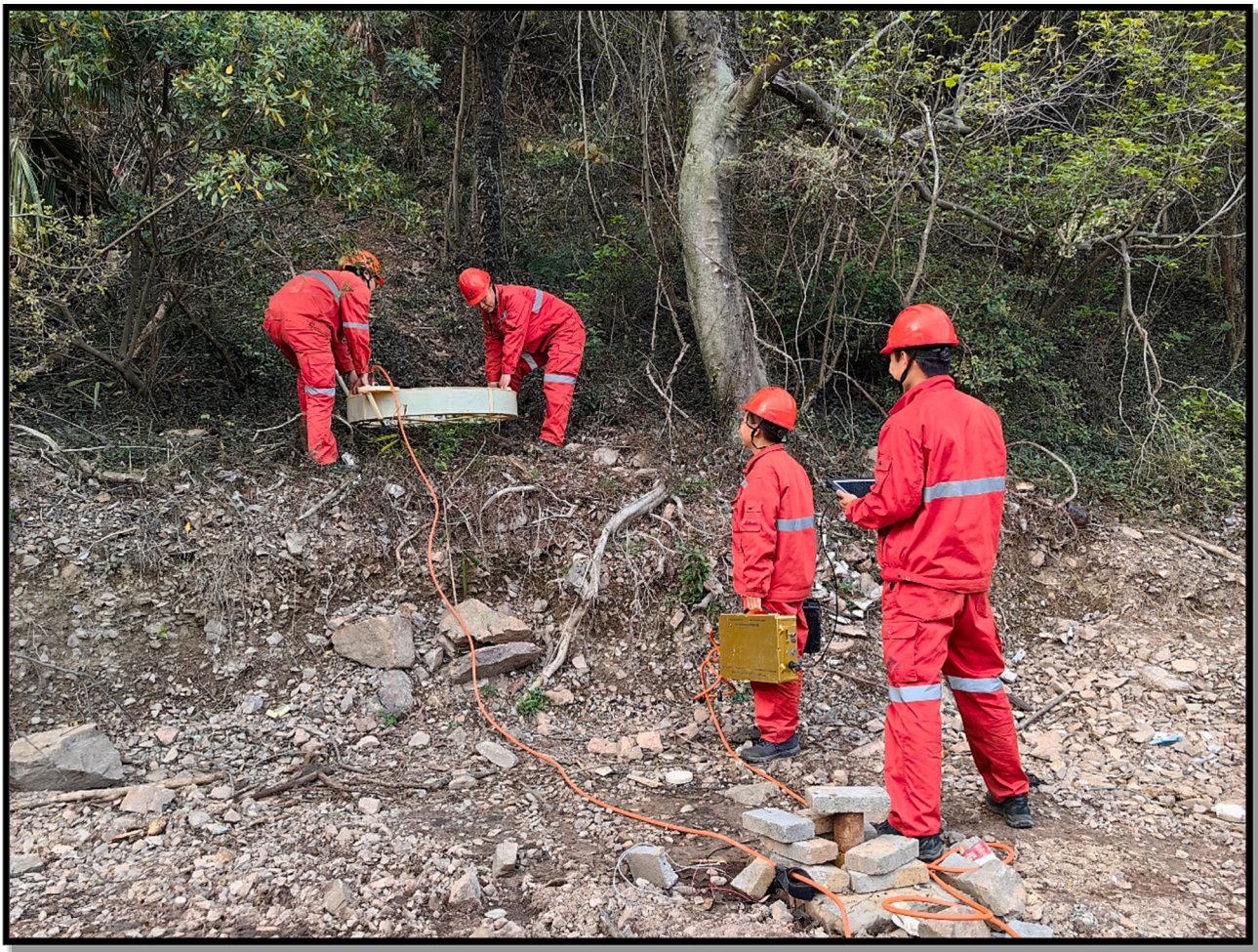
Fig. 1. The small loop TEM system FCTEM used in this study. Inside the white plastic package are the transmitting and receiving coils, and the diameter of the transmitting coil is 1.1 m.
