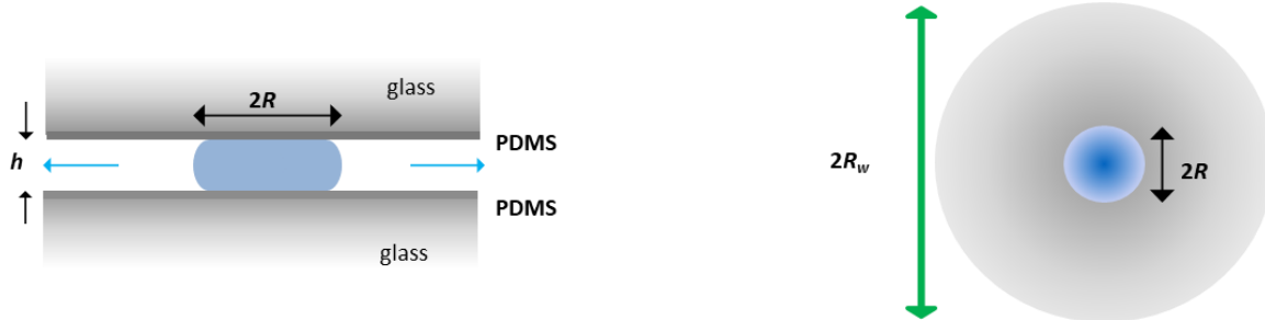
Figure 3. Schematic view of the confined cell for the drying experiment. Left: side view; right: top view.
