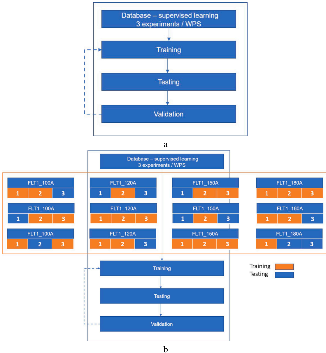
Fig. 12. (a) Data structure for ML. (b) Cross validation example: randomly partition the training and test data into n subsets.
