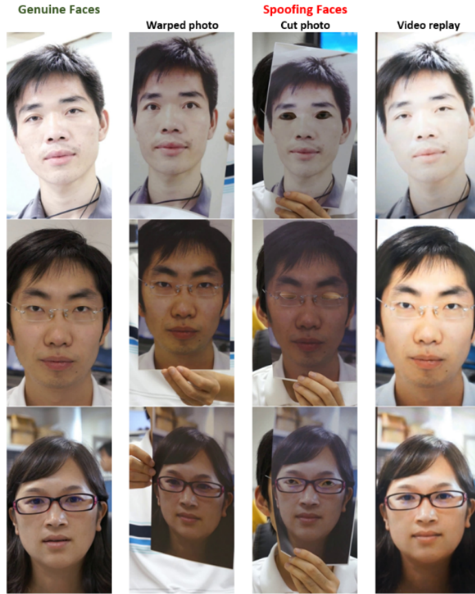
Fig. 8 Live faces and Spoofing faces (Warped photo, Cut photo, and Video replay attacks) examples from the CASIA-FASD dataset
