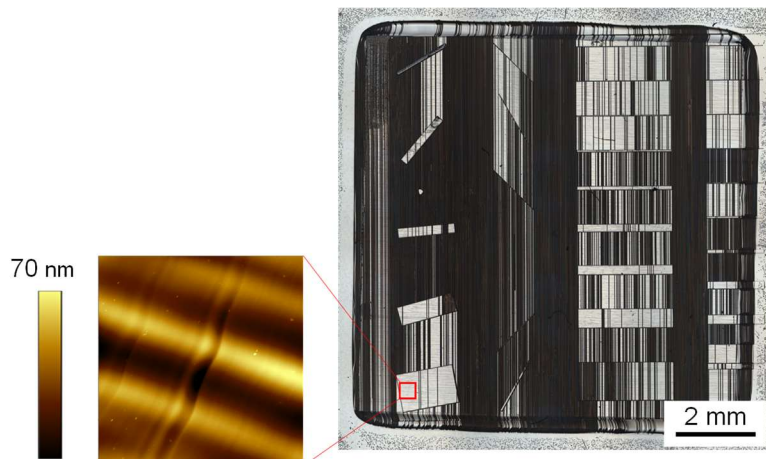
Figure 5. Image of the entire reconstructed area of a B type sample with mesas mostly oriented perpendicularly to the macrosteps edges. This image was obtained by multiple images alignment (MIA) of optical microscope images. The 50 \times 50 \mu\text{m}^2 AFM scan shown on the left was recorded on the red square area of the MIA image.
