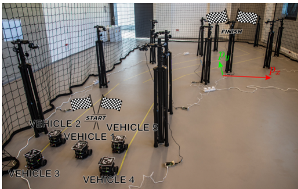
Fig. 8. Distributed formation control with 5 robots in an experiment for research work on distributed state estimation by sensor networks (picture from [15]).
